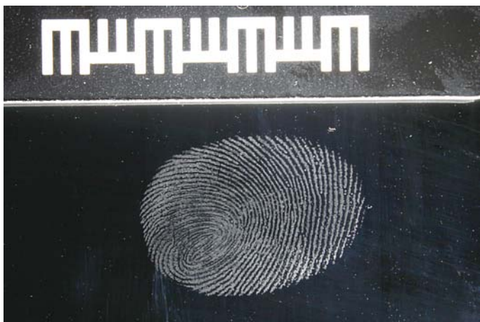
Dark-field illumination of undeveloped latent using the dark-field box
