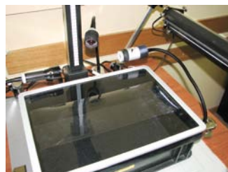
Dark-field box. Before the sample is illuminated with fill-in light
