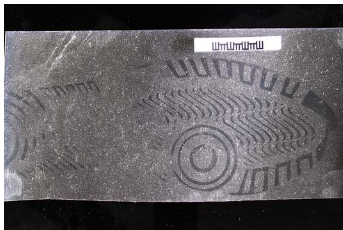
Dark-field imaging of a dust track
